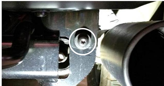
2. Locate the S2 brackets. Using the bolts from step 1 and included spacer, attach brackets on the passenger and driver side in the orientation shown below with spacers under the bracket. Make sure they are level.
