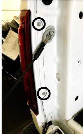
6. With the included Raptor reverse kit upfitter harness in hand, thread the end with a weatherpak plug and an eyelet into the hole behind the tail light and straight down. Make sure the wires exit the body and hang from underneath the vehicle.
